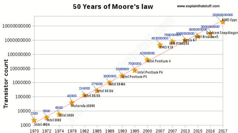
But can the size of transistors continue to decrease from microns (a millionth of a metre) into the realm of nanometres (a billionth of a metre)? The state of current IC technology is often called process. In the table below a 4 micron ( $\mu\text{m}$ ) process refers to the length of the transistor gate.
