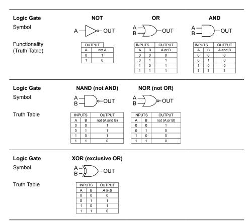
From simple logic gates described below, the components of all computers can be constructed, such as flip-flops and memory components all the way up to ALUs and registers. In fact Arithmetic Logic Units (ALUs) comprise a vital part of the Central Processing Unit (CPU) of a computer. Logical and mathematical operations are performed here. The inputs to the ALU are controlled within the CPU by the control unit.
